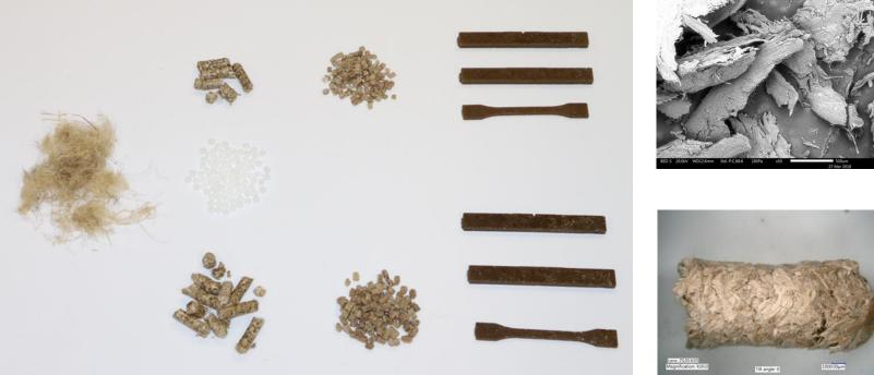
**Thermoplastic Matrixes:** PP, PE, TPE, PA12 ABS, PLA, Green PE, TPS, PCL, PC, POM, PA6,...
